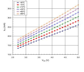
I<sub>cc</sub> versus V<sub>cc</sub> Level Adjust = V<sub>cc</sub>
