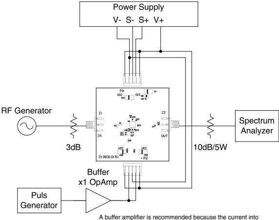
A buffer amplifier is recommended because the current into the Vapc changes with voltage. As an alternative, the voltage may be monitored with an oscilloscope.
