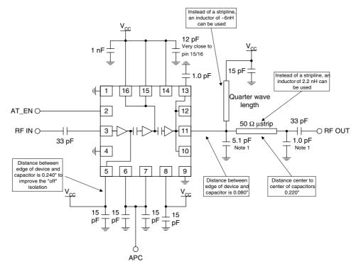
Note: All capacitors are standard 0402 multi layer chip Note 1: Using a hi-Q capacitor will increase efficiency slightly
