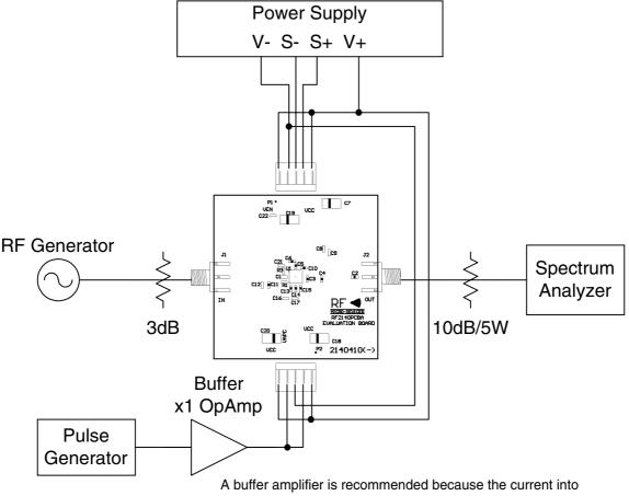
the V<sub>APC</sub> changes with voltage. As an alternative, the voltage may be monitored with an oscilloscope.
