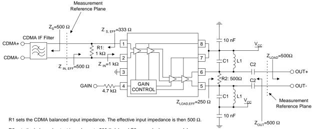
R2 sets the balanced output impedance to 500  $\Omega$ . L1 and C2 serve dual purposes. L1 serves as an output bias choke, and C2 serves as a series DC block. In addition, the values of L1 and C2 may be chosen to form an impedance matching network of the load impedance is not 500  $\Omega$ . Otherwise, the values of L1 and C1 are chosen to form a parallel-resonant tank circuit at the IF when the load impedance is 500  $\Omega$ .
