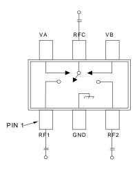
1. DC blocking capacitors not required if negative control voltage is used.
