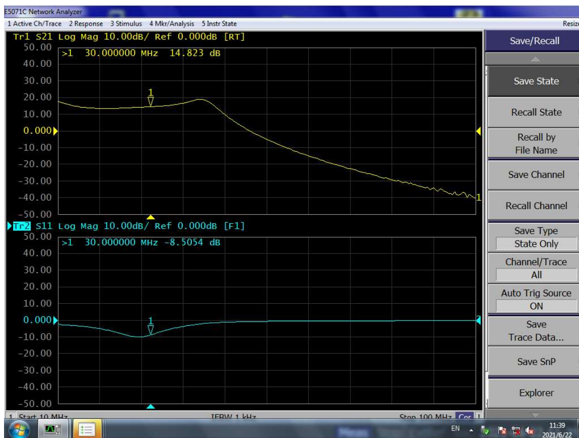
Figure 2: Class C, Low Bias, Low Power Input ( 0 dBm ) S11 / S21
